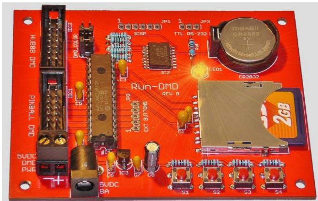
Run-DMD have 4 buttons used for configurations BTN1, BTN2, BTN3 and BTN4 (or S1, S2, S3, S4 with the same functionality).
